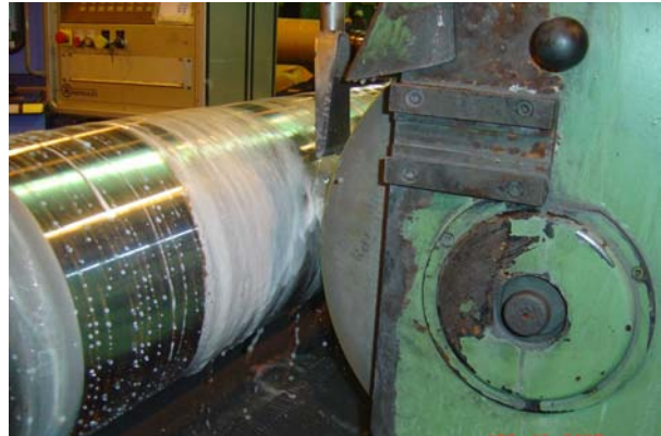
Precision grinding of a steel roll (Photo: OptoSurf)
