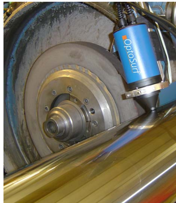
OS 500 Sensor supported on a grinding machine (Photo: OptoSurf)
