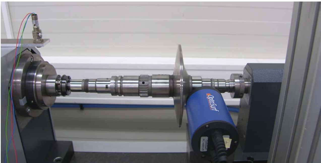
Roundness and roughness measurement on a gear shaft bushing (Measurement IBTL, Kuppenheim)
