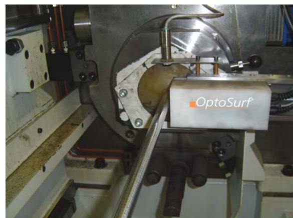
OS 500 measuring in-line during a turning process. The sensor is encapsulated and protected by compressed air against oil mist.
