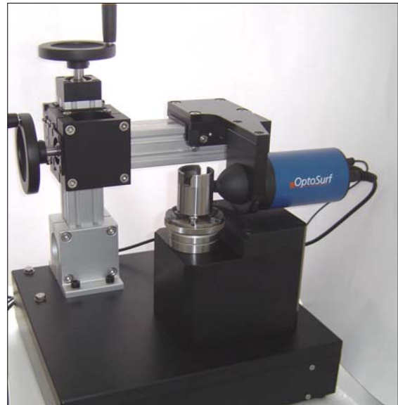
Rotary stage RT1 with OS 500 sensor: Measurement stand with manual z- und x- axis
